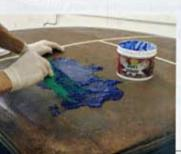
> The bright blue goo worked effectively and quickly. After two applications that were allowed to sit overnight, our rusty roof was stripped down to bare steel nearly everywhere. One more application in the heavy spots and we'd be rust-free.
