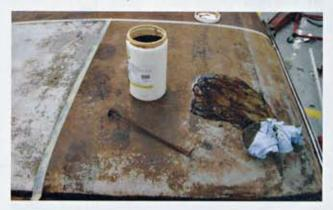
> Just as we suspected, after 12 hours of immersion, the bracket emerged completely rust-free. In cooler weather, this one may be a clinger, but in warm climates, it's best left as a dipping solution.
